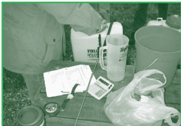
Calibrating a backpack sprayer.
